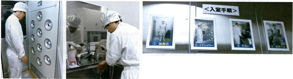
An aseptic room is installed to prevent bacteria from entering sterile drug products during manufacturing process. Many steps of procedures must be followed to maintain the strict level of cleanliness in an aseptic room.
