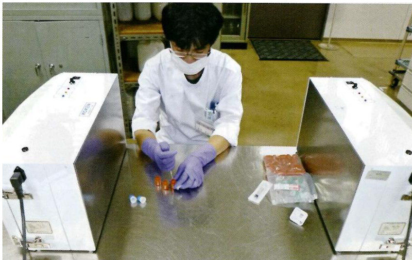
Sterile drug products can be prepared in a clean space formed by the portable KOACH T500-F in a non-aseptic general room.
