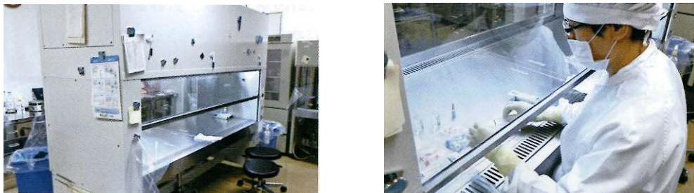
A clean bench is set in an aseptic room. A front glass sliding viewscreen is opened only slightly to prevent contamination.
